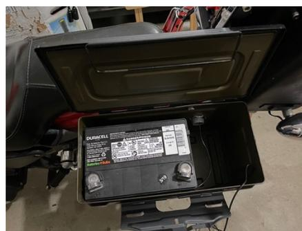
I'm thinking of putting a power panel in the back can on top of the tuner with a few meters, volts, amps & SWR for a manual field antenna tuning option, the fuses, and a main disconnect that I can close to charge the aux battery when the bike is running. The Sporty charge system is crudely rectified 18-20 amps, fine for charging but not so
