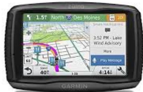
Also, when on battery power, when the battery reaches a certain low level, the display dims to about 40% and cannot be overridden. This is also true of the 396, but not the 660. And at 40%, you'll never be able to read the display during the daytime. And, speaking of batteries, the 595 has a removable battery, the 396 does not.
