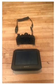
I did some looking at the 396 motorcycle cable and it turns out it's different from previous Zumo cables (550 and 660). Those earlier cables have several wires for power, microphone, speaker, data etc. The cable for the 396 only has 2 wires. If you look at the contacts between the mount and the device (2 little brass pins), there are only 2 contacts. So, I assumed those would only be power. I assumed correctly – and it turns out it's only 5v power. Looking at the original Garmin cable
