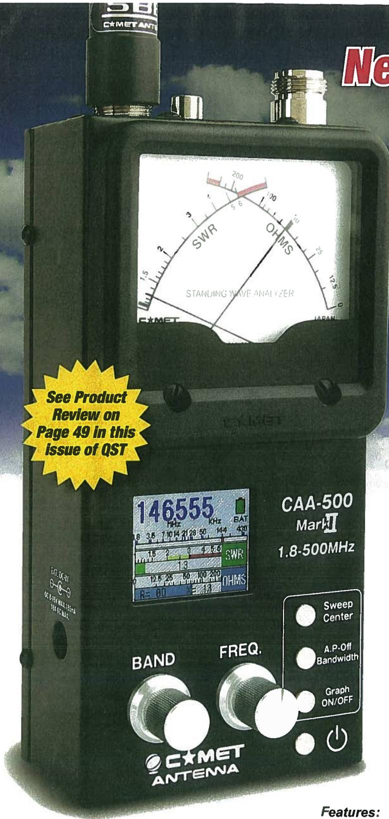
The perfect combination of analog and graphic information, designed in particular for antenna diagnostics and adjustments while on the roof, tower or in the field!
